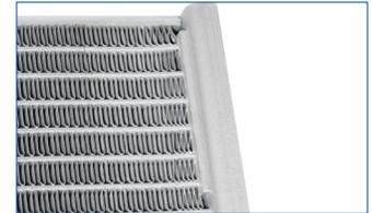
Flex-A-Lite® Extruded Tube Core Radiators include a corner subhead, reinforcing the cooling tube to header connection; an area prone to cracking and leaking in other brands of radiators.
