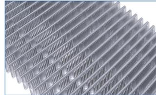
The cooling fins have been designed with specific louver patterns punched into them to direct airflow, increasing heat rejection and providing better cooling performance.
